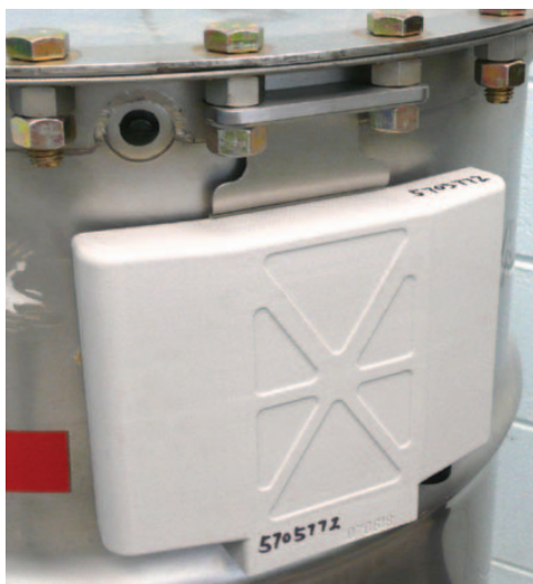
3 Left: prototype tag mounted on Model 9975 drum and right: interior view of tag with metal back plate removed
